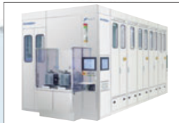
Batch-type cleaning equipment
