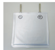
Lithium-ion battery prototype, with laminated pouch structure
